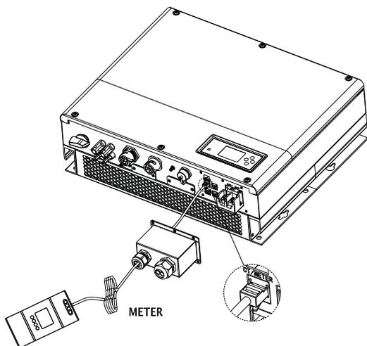
e. Connect the A+ of RS485 cable to Pin7 and B- of it to Pin8.
