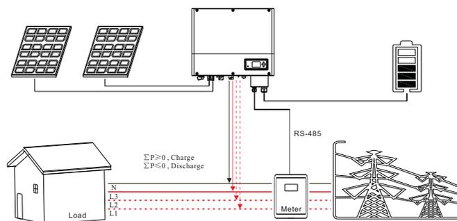
c. Install the three-phase energy meter in inlet AC distribution cabinet, and connect it to the utility grid (L1, L2, L3) according to responding indicator mark. The arrow on the meter indicates the grid access port.
